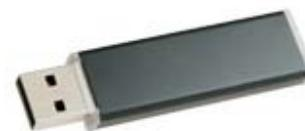
Removing the disk is easy. Simply pull it out of the port. There is no "Safely Remove Hardware" icon to click.
