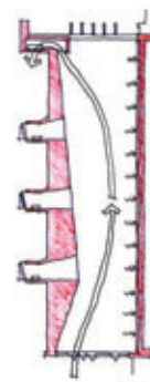
Mode 5. Peak Cooling Events. Minimum outside air. Cool space using chilled water in radiant slab from backup heat pump.
