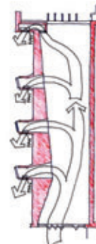
Mode 4. Cooling Season. Maximum air movement via roof fans. (Skylights are closed.) Use of "night purging" using natural ventilation with cool night air.
