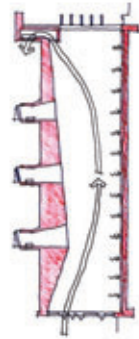
Mode 5. Peak Cooling Events. Minimum outside air. Cool space using chilled water in radiant slab from backup heat pump.
