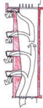
Mode 4. Cooling Season. Maximum air movement via roof fans. (Skylights are closed.) Use of "night purging" using natural ventilation with cool night air.
