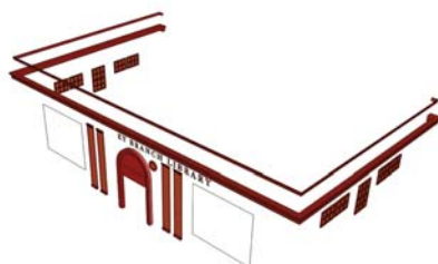
West portion of text 'WEST BERKEL' has been damaged by construction of addition; East portion of text 'EY BRANCH LIBRARY' in good condition
